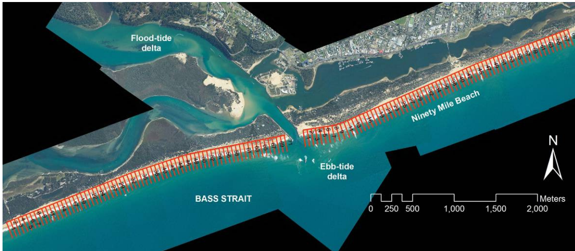
Figure 5. Positioning of east and west transects adjacent to the Gippisland Lakes artificial entrance to monitor sandy barrier shoreline changes.
