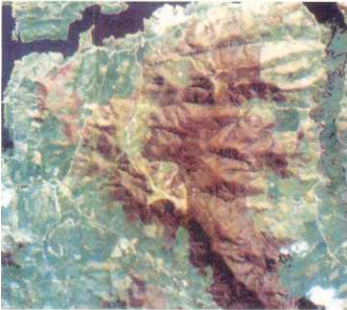
Figure 2. A linear contrast enhanced sub-scene of a TM image after geometric registration. The purple tones depict the distribution of (flowering) Paterson's Curse but only for areas more densely infested. The area documented on one of the archival ground photographs taken within a few days of the imagery is indicated by the broad arrows. Small arrows indicate the location of Tallangatta. The image is from the scene: Path 91, Row 85, 29/10/88.
