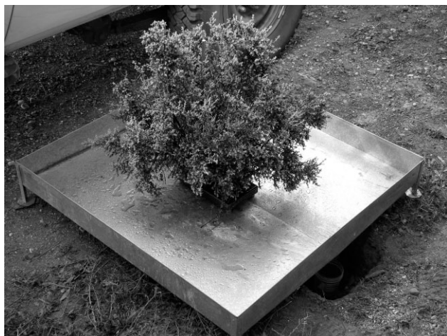
Figure 2. A bluebush shrub in test position on the throughfall tray. The outlet pipe is concealed behind the front wall of the tray, but the runoff collecting container can be seen in the small pit at the lower right of the image. The tray measures 1 m × 1 m
